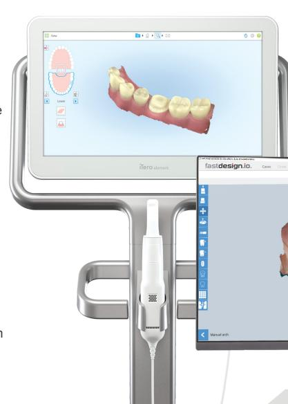
for the restoration, which the dentist can accept or revise according to preference. From the same software interface, the dentist can either prescribe and request a restoration from Glidewell Laboratories, or send the design direct to the fastmill.io In-Office Unit for immediate chairside milling.
