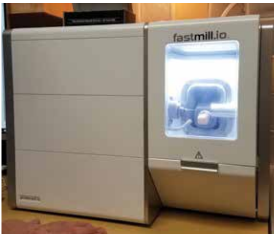
Figure 15: The BruxZir NOW crown was milled in less than 40 minutes with the fastmill.io In-Office Unit.
