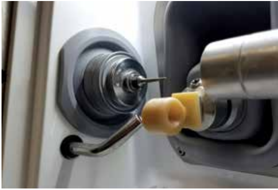
Figure 14: A torque wrench was used to secure the BruxZir NOW zirconia block to the fastmill.io unit for fabrication of the crown.
