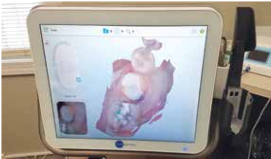
Figure 6: After completing the digital impression, the iTero Element scanner converts the scans into a virtual model. Note that any missing data is flagged with color coding so the area can be rescanned and incorporated into the digital model. Once the virtual model is generated, the clinician can easily evaluate, rotate and magnify the model for evaluation of the scan and tooth preparation.
