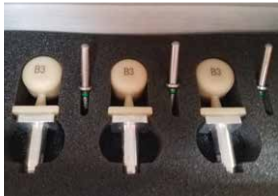
Figure 13: The BruxZir NOW zirconia milling blocks are pre-shaped in cylindrical form to minimize fabrication time. The blocks are also fully sintered, which eliminates the step of using an oven to sinter the zirconia before delivering the dental restoration.
