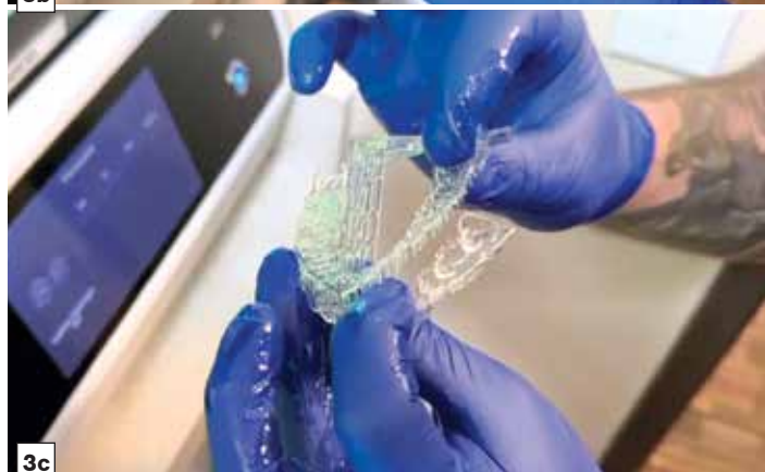
Figures 3a–3c: 3D-printed retainers are removed from the print plate, then separated from the supports.
